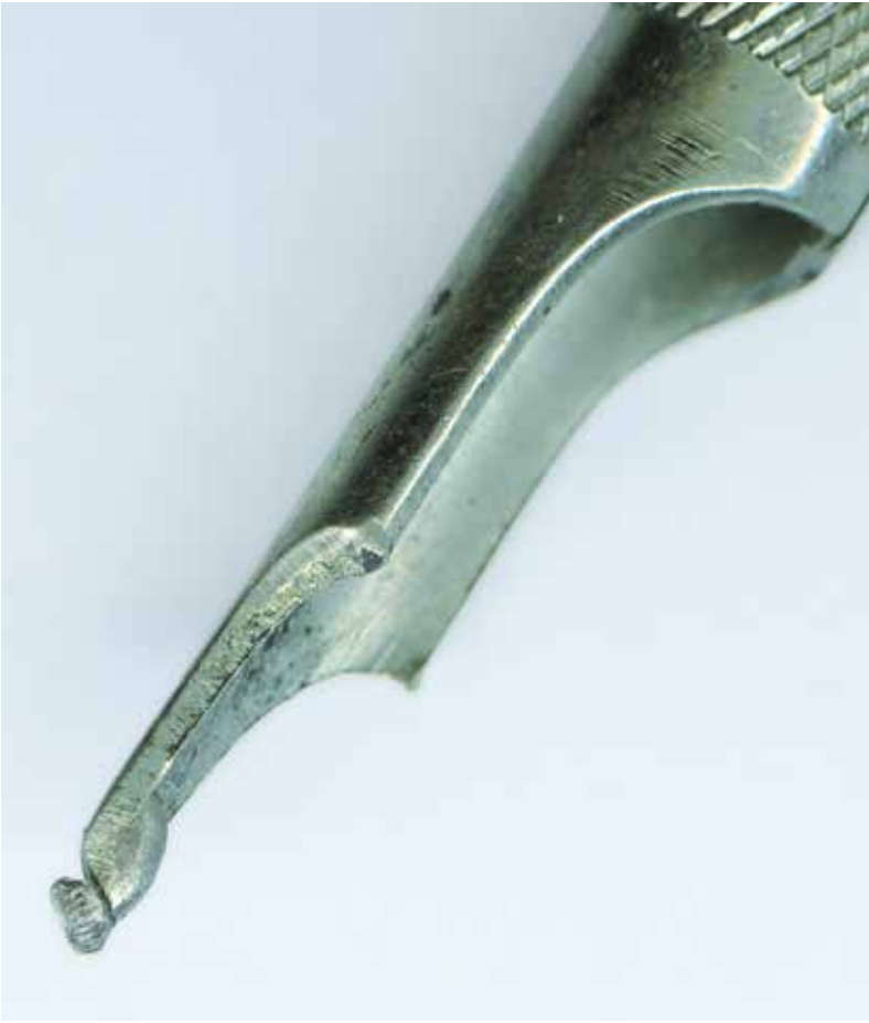
Gestetner's stencil paper. Neo-Cyclostyle pen with perforating wheel.
