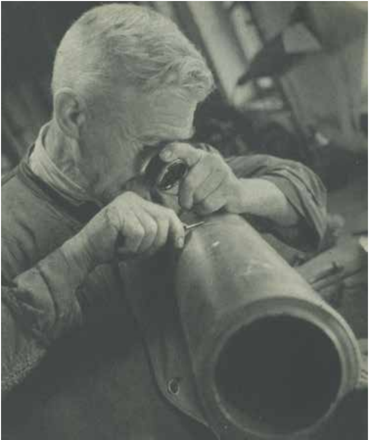
ABOVE: Working with the Pan-tograph. The enlarged version of the design is transferred onto the printing cylinder at a reduced size and engraved on the cylinder surface with a diamond point. USA, ca. 1923.
